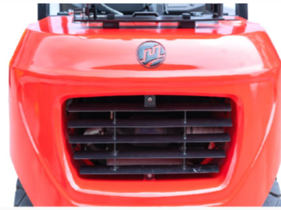
Add counterweight grill, effective dustproof and internal protection, increased safety
